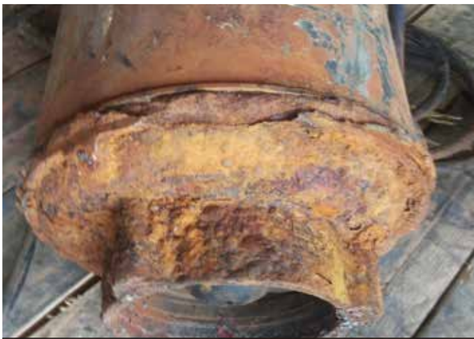
Without sacrificial anode : 5 months pumping in seawater applications
